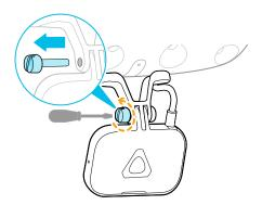
2. Release the sensor unit from the frame. Rotate the cable clip to a horizontal position to unlock, and slide horizontally. Finally, unplug the USB cable from the headset.
