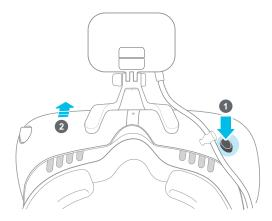
Step 4: Connect the tracker cable to the headset
