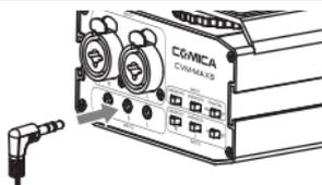
➡ For mono mic, connect it to the corresponding 'L' / 'R' input jack
