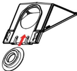
2. Install the adapter ring with foam on the adapter
