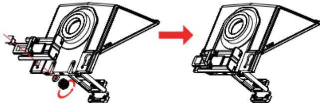
4. Unscrew the knob from the smartphone holder. Smartphone holder can be installed on either side depending on your preference. To record horizontal footages install smartphone holder vertically. To record vertical footages install smartphone holder horizontally
