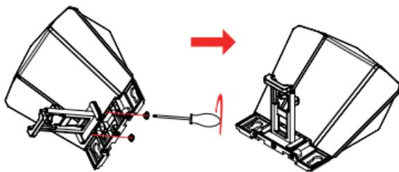
2. Use the included screwdriver to attach the phone clamp
