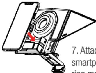
7. Attach the phone to the smartphone holder. Foam ring may need to be rotated and adjusted for various smartphone camera locations
