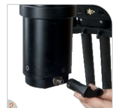
Air-pressure in the pneumatic column can be adjusted
