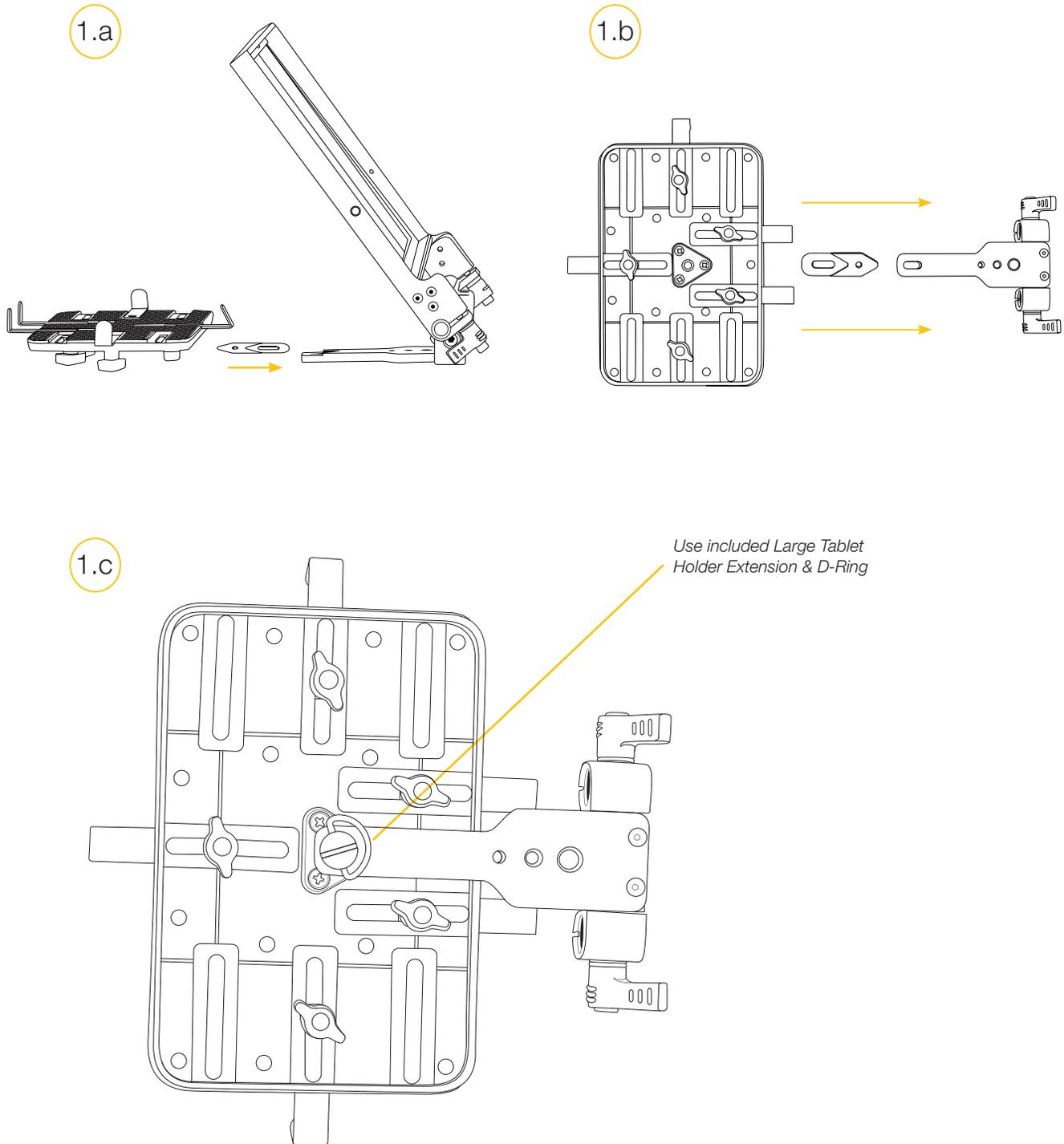
Tighten & loosen thumb screws to adjust glass frame. Ideal angle is 45 degrees.
