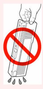
• Put the used one immediately into the plastic bag attached to the new maintenance cartridge and seal the bag by tying the opening tightly to prevent the ink from leaking.
