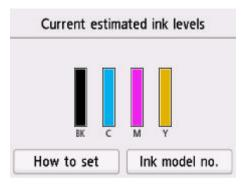
When the ink level is low, is displayed above the ink level on the touch screen, and is displayed when ink runs out.
