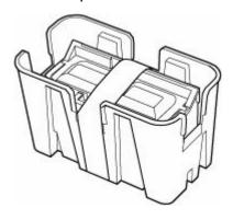
**11.** Remove tape used to secure print head.
