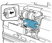
8 Push the roller lock lever up to lock the feed roller.
