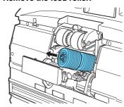
6 Place the new feed roller on the pin.
