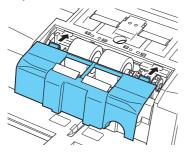
Push the front of the retard roller cover in. Make sure that the front unit is completely closed by pushing until you hear a click.
