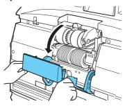
3 Pull the roller lock lever down.
