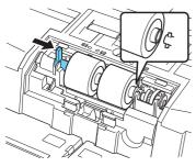
Pull the roller lock lever down to lock the retard roller in place.
