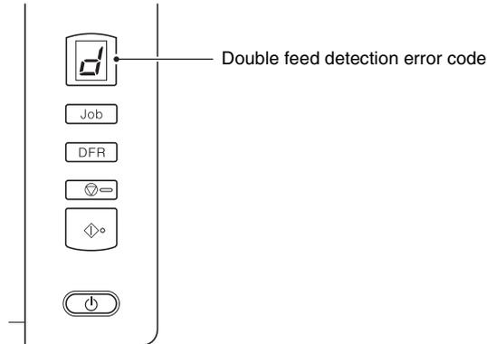
Also, a message screen is displayed to notify you that a double feed has been detected. For example, the following screen is displayed in CapturePerfect.
