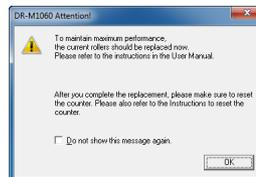
If this message begins to be displayed at startup, purchase an exchange roller kit and replace the worn parts with the consumable parts included in the kit (feed roller and retard roller). See p. 85 for details about the exchange roller kit.
