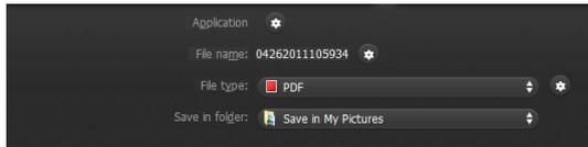
Saves the scanned image file in a specified folder and then opens it with a specified application. When you specify this output method, click the [Application] button and specify the executable file of an application that can open image files. In addition, configure the settings of the image file to be saved
