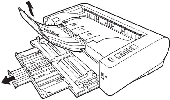
**5 Adjust the document guides to fit the width of the document to be scanned.**
