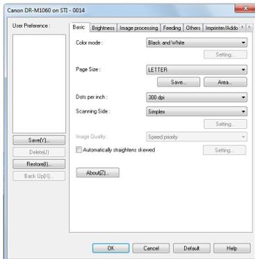
Configure basic scanning conditions such as the mode, page size, resolution, and scanning side. In addition, you can click the [Area] button and specify the area to be scanned.
