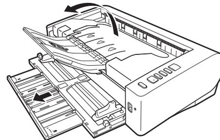
When scanning documents longer the LTR horizontal (216 mm), extend the feed support and eject support extensions.
