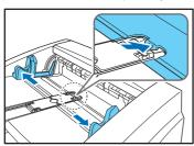
When closing the imprinter cover, make sure that it is locked so that will not open unexpectedly. An error message appears on the display panel if the imprinter cover is open.
