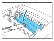
**10.** Press down on the tab of the imprinter cover (as indicated by the arrow in the illustration) to lock it.
