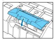
6. Carefully lower the upper unit (1). Press down on both sides of the upper unit to ensure that it is securely closed. (2)
