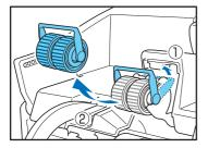
**4.** Pull the feed roller lock lever down (①) and move it to the right (②) to unlock the feed roller.
