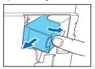
Peel off the seal covering the nozzles of a new ink cartridge.
