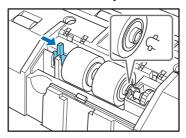
**3.** Pull the roller lock lever down to lock the retard roller in place.
