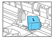
**6.** Peel off the seal covering the nozzles of a new ink cartridge.
