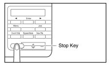
Each time you press the Stop key, the upper and lower platen rollers rotate in the following order: black → white → brush
