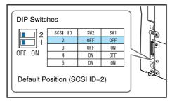
The DR-X10C II scanner incorporates a SCSI terminator which is permanently set to ON. When using a daisy-chain configuration with other SCSI devices, make sure that the DR-X10C II scanner is connected as the last device in the chain. Set the terminators of all other devices to OFF.
