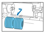
6. Use a moistened, well wrung-out cloth to wipe off any dust from the rollers.
