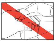
Lift the pickup roller mounting lever, and remove the roller.
