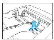
• To reset the guides so that they are equidistant from the center, spread the guides all the way to the left and right.
