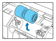
Use a moistened, well wrung-out cloth to wipe off any dirt from the roller.
