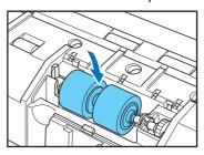
2. Align the notches in the roller with the shaft pins in the scanner, then slide the roller lock lever in the direction indicated by the arrow.
