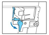
3. Open the carriage and remove the ink cartridge.
