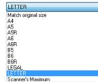
If [Match original size] is selected, the edges of the document are detected and images that match the size of the document are saved. Further, [Trimming] in the [Image processing] tab is enabled only when [Match original size] is selected.
