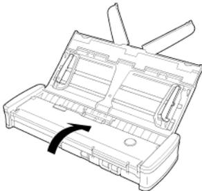
After you remove the jammed paper, check to see if the last page was scanned correctly, and then continue scanning.
