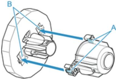
5. Insert holder stopper from left into Roll Holder as shown, and while holding in position (B), push firmly until holder stopper flange (A) touches roll paper. Lift holder stopper lever (C) from shaft to lock.
