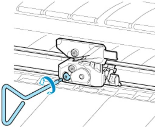
7. Remove cutter blade while holding D.
