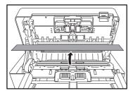
6. Remove the stopper and sheet from the feed roller.
