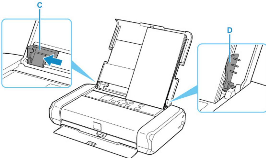
Fold flap of the envelope and load the envelope in portrait orientation with the address side facing up.
