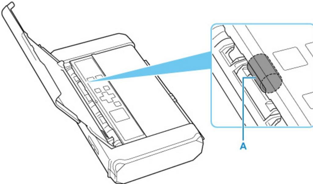
After cleaning the paper feed roller with a cotton swab, turn on the power, then clean the paper feed roller again.
