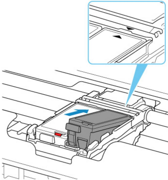
6. Press the PUSH mark on the ink tank until the ink tank snaps firmly into place.
