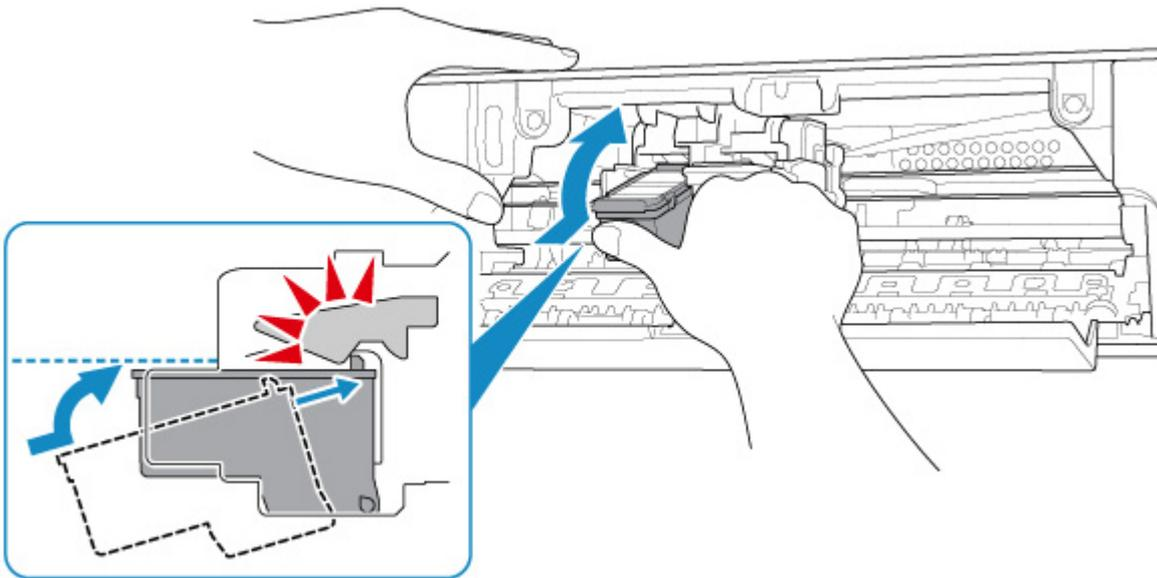
After confirming that the FINE cartridge is installed properly, close the cover.
