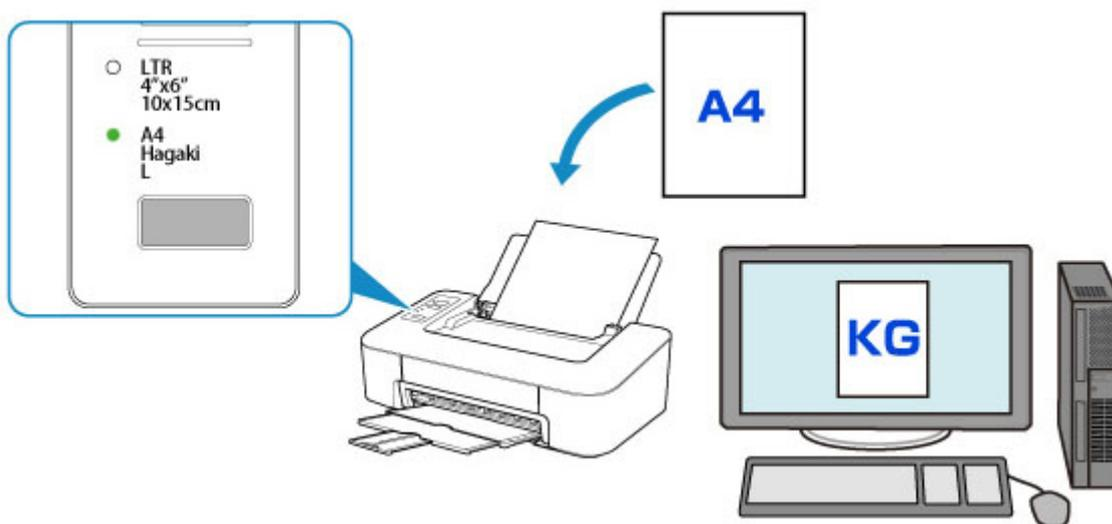
When you start printing, the **Alarm** lamp and the **Paper** lamp indicating the paper size setting for printing flashes in synchronization.
