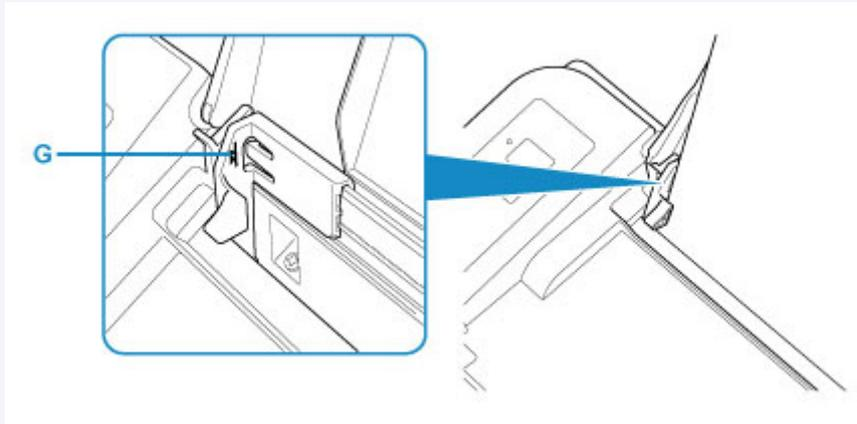
After loading paper on the rear tray, either of the **Paper** lamp lights up according to the paper size loaded last.
