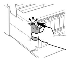
9. After you replace all the cartridges that need replacing, close the printer cover.
