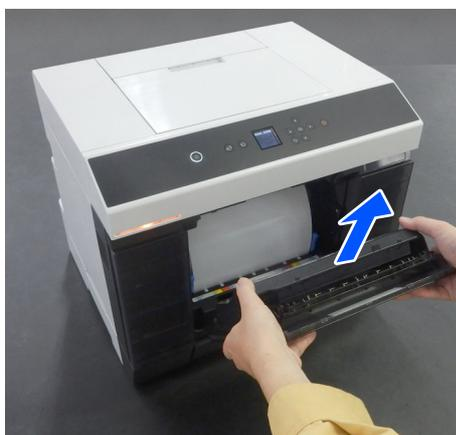
When the scrap paper box is removed, the status light lights.
