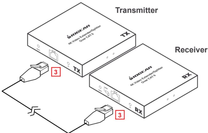
**NOTE:** It is recommended to use a network cable with a length between 7 and 230 feet. If the cable is too short, there may be no display output because the signal is too strong. If the cable is too long, the output may have poor quality.
