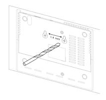
Insert the supplied two Anchors into the wall. If necessary, use a small hammer to lightly tap the anchors flush to the wall.
