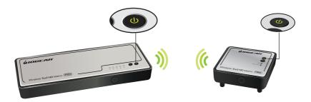
3. During start-up, the **Source LED indicators** on the Transmitter and the **Wireless Signal** status LED on the Receiver will flash green until the signal link has been established with the Transmitter. This process takes approximately 30 seconds.
