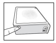
1. Open the ribbon door by pushing the ribbon door switch
