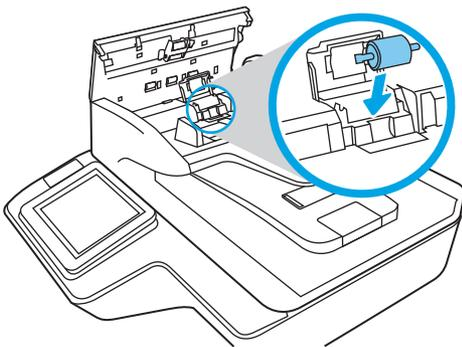
5. Replace the roller cover, and then continue with replacing the pick up roller module.
