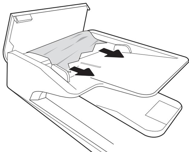
4. Lift the scanner lid and remove any jammed paper from the bottom of the scanner lid.
