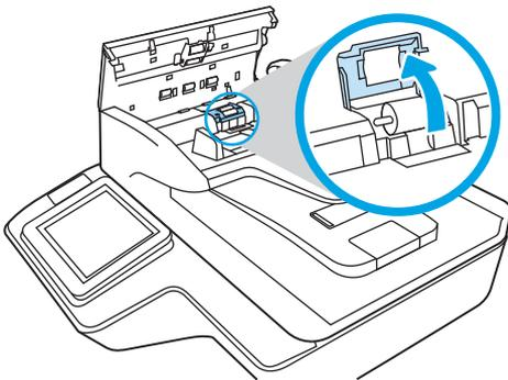
4. Remove and replace the rollers as described in the instructions included with the replacement kit.
