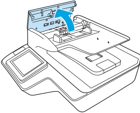
3. Squeeze the tabs on the sides of the roller cover, and then lift up the roller cover to remove.
