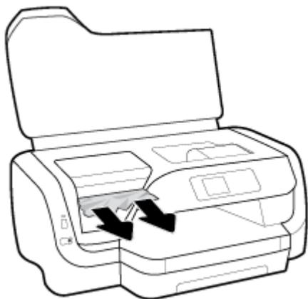
3. If need, move the print carriage to the leftmost end, and remove any jammed or torn pieces of paper.
