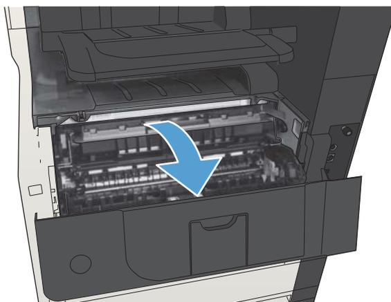
2. Grasp the handle of the used toner cartridge and pull out to remove.
