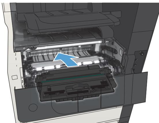
8. Close the cartridge door. After a short time, the control panel should display the **Ready** message.
