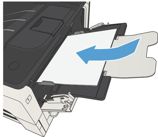
6. Adjust the paper-width guides so that they lightly touch the paper stack but do not bend the paper.
