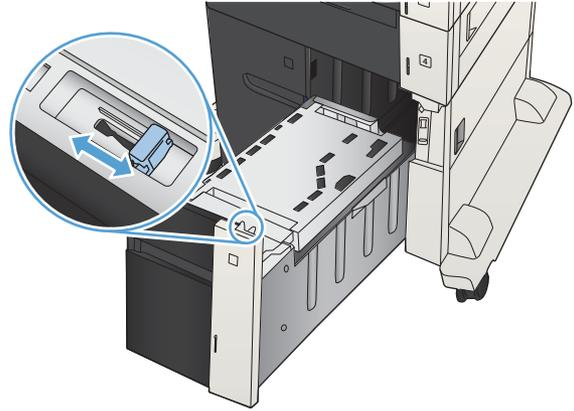
3. Load full reams of paper into each side of the tray. The right side holds 1,500 sheets of paper. The left side holds 2,000 sheets of paper.
