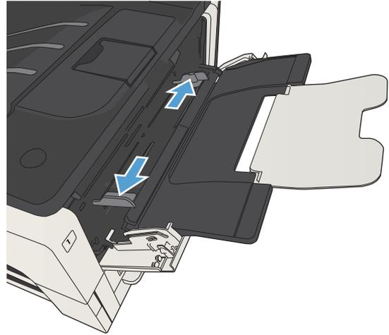
5. Load the paper into the tray. Make sure that the paper fits under the tabs and below the maximum-height indicators.
