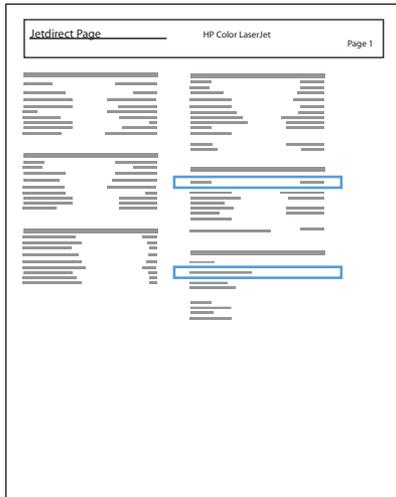
5. **IPv4:** If the IP address is 0.0.0.0, or 192.0.0.192, or 169.254.x.x, you must manually configure the IP address. Otherwise, the network configuration was successful.
