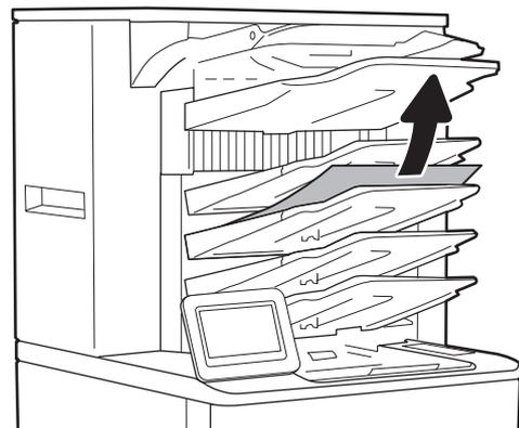
2. Open the jam-access door on the back side of the stapling mailbox. If jammed paper is visible inside the jam-access door, pull it straight up to remove it.
