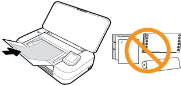
3. Slide the paper-width guides inward until they stop at the left and right edges of the paper.
