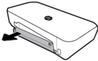
4. If you are replacing the battery, remove the original battery by lifting the latch and releasing the battery.
