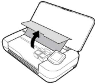
2. Remove all visible paper by moving the cartridges around from one side to the other.
