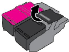
4. Remove the protective film from a new cartridge.
