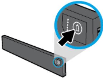
**TIP:** If the battery is installed in the printer, press similar button on the battery cover.
