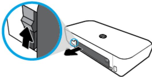
5. Insert the battery into the battery slot.
