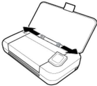
3. Insert the envelope print-side up and the long-edge flap on the left or the short-edge flap at the top.
