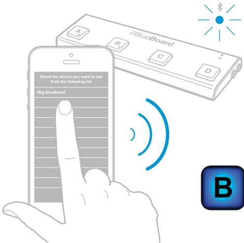
In this mode iRig BlueBoard communicates with the control app (iRig BlueBoard) and the Control app converts the data to standard MIDI messages.
