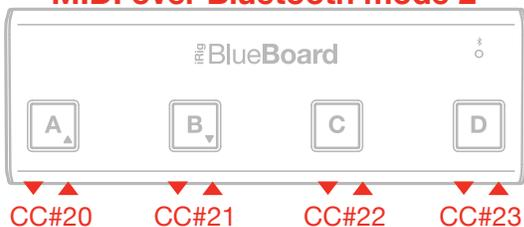
In MIDI over Bluetooth mode 2, iRig BlueBoard sends MIDI Control Changes when the A, B, C and D foot switches are pressed.
