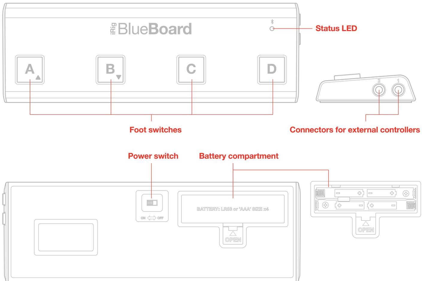
iRig BlueBoard is equipped with four backlit soft-touch pads housed in a sturdy, stageworthy chassis, two TRS jacks for connecting additional controllers like foot switches and expression pedals, and is powered by four standard AAA batteries.
