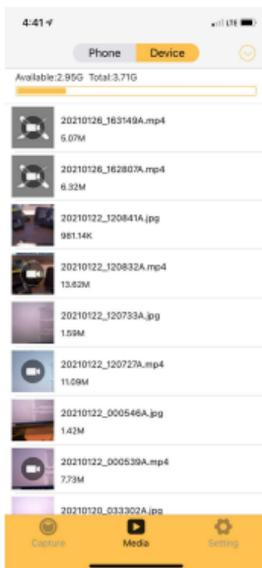
To download media to your smartphone or to delete media from the camcorder, press the down arrow at the top right corner of the smartphone screen. Then select Download or Delete. Select the media you wish to download or delete and tap the confirm button on the bottom right corner of your smartphone screen. If a photo or video is deleted on the app, it will also be removed from the SD card in the camcorder.
