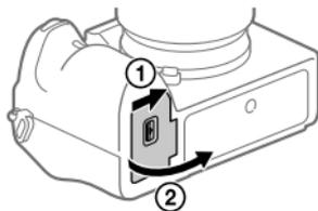
**2** Insert the battery pack while pressing the lock lever with the tip of the battery until the battery locks into place.
