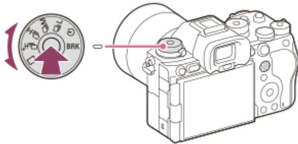
Turn the drive mode dial while holding down the drive mode dial lock release button in the center to select the desired mode.
