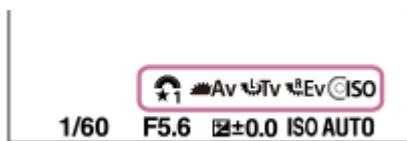
2. Turn the control wheel to set the ISO value, turn the front dial to set the aperture value, turn the rear dial L to set the shutter speed, and turn the rear dial R to set the exposure compensation.
