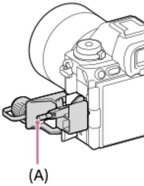
3. Push in the attachment screw **(A)** and turn it to secure the cable protector.
