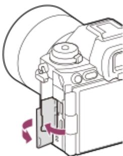
2. Attach the cable protector as illustrated so that it fits the shape of the terminal surface of the camera.
