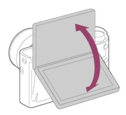
You may not be able to adjust the monitor angle depending on the type of a tripod you use. In such a case, release the tripod screw once to adjust the monitor angle.
