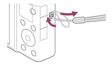
To use a shoulder strap (sold separately), attach the strap adaptors (supplied) to the strap hooks on either side of the camera.
