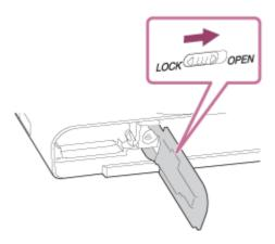
Insert the battery pack while pressing the lock lever (A) with the tip of the battery until the battery locks into place.
