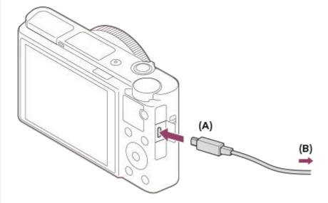
**A:** To the Multi/Micro USB Terminal **B:** To the USB jack of the computer
