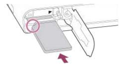
With the notched corner facing in the direction illustrated, insert the memory card until it clicks into place. Insert the memory card correctly. Not doing so may cause a malfunction.
