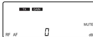
It shows the microphone input sensitivity is now at 0dB (default setting).
