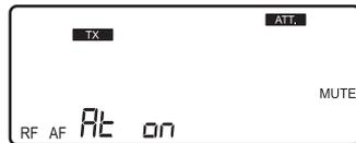
The function is activated with 20dB of audio input attenuation.
