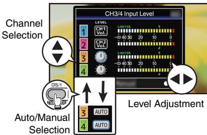
**3 Press the Set button (●) to end the adjustment.**
