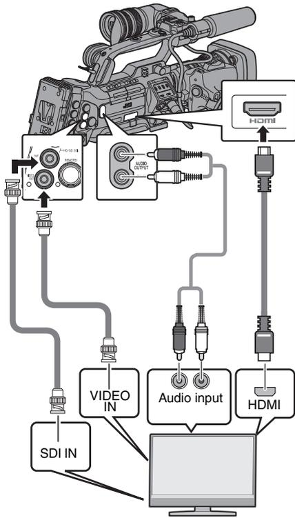
\* Select the output signal in [A/V Set] → [HDMI/SDI Out].
