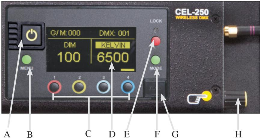
**A) On /Off:** **On** = Green light displayed. **Off** = Red light displayed. The display and all menu settings can be operated while the power button is in the **Off** position, as long as power is applied to the fixture. The On /Off button only controls the light source.
