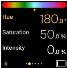
The *Adjustment Dial* ⑤ cycles through colors from the color wheel. Due to display space constraints, this wheel is represented as a horizontal color bar at the top. The display indicates the corresponding hue angle from the color wheel in degrees.
