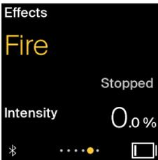
The purpose of the *Effects Mode* is to be able to start and stop effects directly from the Play. Each effect has multiple settings and parameters. The parameters of the various effects are adjusted in the Kelvin Narrator App, and the Play will keep these settings until changed again in the app.
