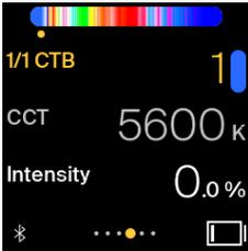
The Kelvin Play offers a diverse array of digital gel filters. With *Filter Mode*, matching the color temperature of nearby lights is straightforward. Once aligned, any of the available digital gels can be selected to add a hint of color for background illumination or as an accent light. Each gel is numbered and titled and features a color bar of the color hue and the exact color temperature.
