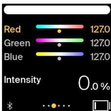
Use the *Function Button* ③ to select which parameter to adjust, and the *Adjustment Dial* ⑤ to change the value. The color bar at the top shows the resulting color.
