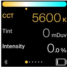
The dials adjust brightness, color temperature and tint. Brightness is adjustable from 0.0 to 100.0%.
