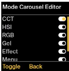
The *Mode Carousel* is customizable, allowing for quick access to selected modes. Modes that are toggled 'ON' will appear in the list when you press the *Mode Button* ② later.
