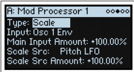
This processor uses a modulation source to scale the input. For instance, you can control the amount of an LFO with an Envelope, or control the amount of an Envelope with a MIDI controller.
