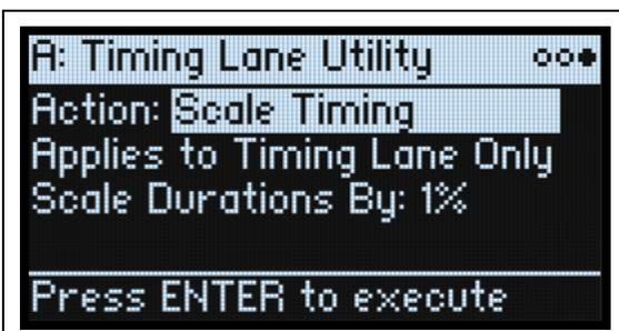
This Action is available only when entering the Motion Sequence Utility page via the Timing Lane. It allows you to edit all of the Timing Lane Step Durations at once, to make the sequence longer or shorter. If you want to change this in real-time, use the Timing Lane **Speed** parameter instead.
