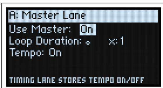
When **Use Master** is *On*, the Master Lane restarts all of the other Lanes after either a specified number of beats or elapsed time, depending on the **TEMPO** On/Off setting. You can use this to create regularly repeating patterns, even if the different Lanes all have irregular loop lengths.
