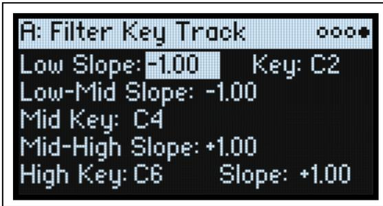
Most acoustic instruments get brighter as you play higher pitches. At its most basic, keyboard tracking re-creates this effect by increasing the cutoff frequency of a lowpass filter as you play higher on the keyboard. Usually, some amount of key tracking is necessary in order to make the timbre consistent across the entire range.
