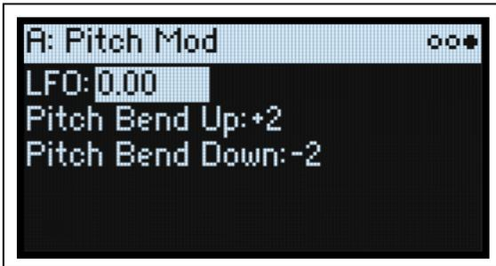
These settings apply to the entire Program, including Osc 1/2 and the Sub Oscillator. To modulate the pitches of individual Oscillators, use the Osc Pitch page instead.
