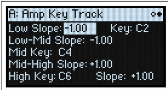
Keyboard tracking (“Key Track”) changes the volume as you play up and down the keyboard. This may be used to make the volume more consistent, or to create special effects.
