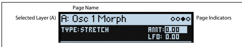
**LAYER A/B:** Layers contain a Program, an Arpeggiator, and a handful of other settings. The front panel edits one Layer at a time, as selected by these buttons. To turn a Layer on or off, hold **SHIFT** and press the Layer’s button, or just double-press the button.
