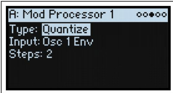
This changes a continuous signal into a series of discrete steps. Use this to change the shape of LFOs or envelopes, or to force a controller to land on a few specific values.
