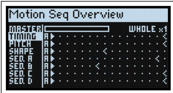
This shows all of the Motion Sequence Lanes for the Layer’s oldest sounding voice. It displays up to 16 steps at once, matching the 16 front-panel buttons, for each Layer. The bank, A/B/C/D, is shown to the left of the steps. For each lane, the display automatically shifts to show the bank containing the active step.
