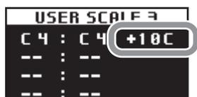
Turning the PROGRAM/VALUE knob while holding the SHIFT button will shift the note name played to an entirely different note.
