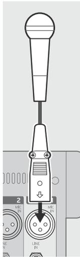
**5** Plug a microphone or other audio source into the first channel's rear panel **MIC IN** socket.
