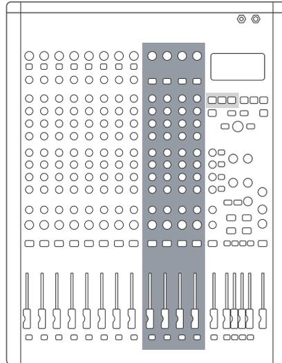
Stereo channels have a few different controls and many identical ones.
