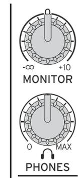
The monitor output will output either the **MAIN L/R** bus or the monitor bus. The signal source is indicated by the **CUE** indicator.
