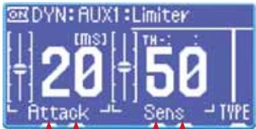
A limiter is basically a very fast compressor with a very short attack and a moderately short release. *Attack* controls how fast the limiter takes to react; *Sens* (sensitivity) determines how intense a signal it reacts to.
