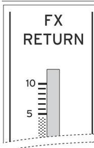
**FX RETURN** fader adjusts the volume of the effect sent to the **MAIN L/R** bus.
