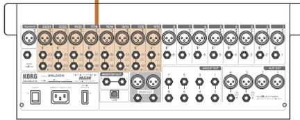
devices such as DVD players or feeds from a laptop (the balanced mono XLR **MIC IN** jack on each stereo channel is for connecting a mono microphone only).
