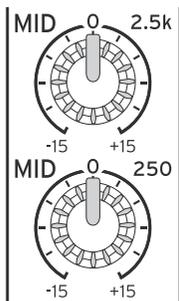
Stereo channel MID equalization consists of two controls with fixed band centers: 2.5kHz high Mid and 250 Hz low Mid.
