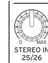
Adjusts the volume of the front panel **STEREO IN** jack.
