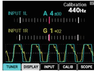
You can set the reference pitch to a value other than 440 Hz (this is also called “concert pitch,” meaning a range from middle C to the A below that). With this function, you can tune multiple oscillators at the same time by transmitting the same pitch (note) and adjusting the pitch while monitoring.
