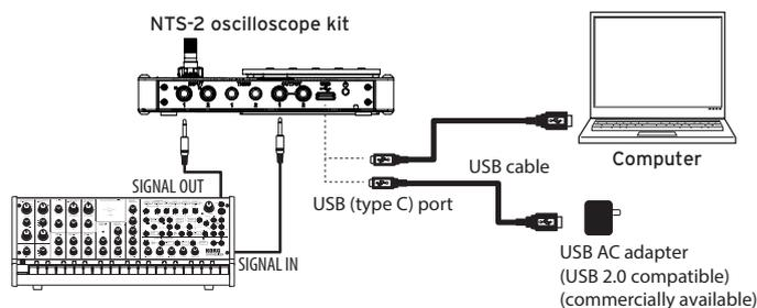
Use the included USB cable to connect this unit to the USB port on your computer or to a commercially available USB standards-compliant AC adapter (at least 5 V DC 550 mA).
