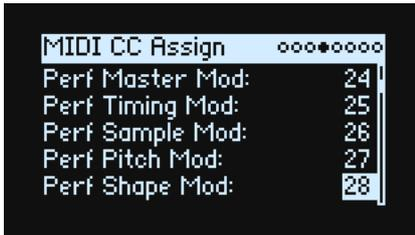
You can control Scale Select and each Mod Knob directly from MIDI CCs. These CCs edit the assigned parameters, just like moving the front-panel knobs. To modulate a parameter with variable intensity, and without causing edits to the sound, use modulation instead. Some dedicated CCs cannot be assigned (CCs 1, 7, etc.).
