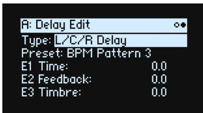
The **EDIT 1/2/3** controls (E1/E2/E3 on the display) are macros which may control multiple internal parameters, and which may be set up differently for each **Preset**. There are general conventions for the **EDIT** knobs of each effect **Type**, as reflected in the on-screen labels.
