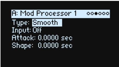
This creates more gentle transitions between values, smoothing out abrupt changes such as a quick move on a wheel or a sharp edge on an LFO.
