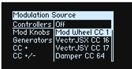
6. Use **<** and **>** to move between the columns, and **VALUE** to select items in the lists. Alternatively—and faster!—most modulation sources can be selected by pressing their associated front-panel button (for Envelopes, LFOs, and the Step Sequencer), or by holding down **ENTER** and moving a controller (such as a Mod Knob, wheel, or the Vector Joystick), playing a note on the keyboard (for Velocity), or sending MIDI data.
