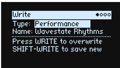
2. To choose a different data type, hold **WRITE** and press a button such as **LAYER A/B/C/D** (for Programs), **SET LIST**, or **WAVE SEQUENCE**, or set the Type manually in the display.
