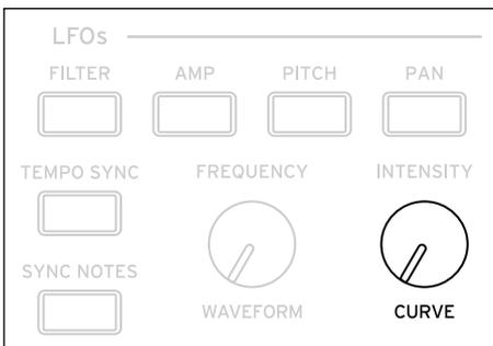
**Curve** adds curvature to the basic waveform. As you can see in the graphic below, this can make the waveforms either more rounded or more extreme. It can also be useful to emphasize certain value ranges, and deemphasize others.
