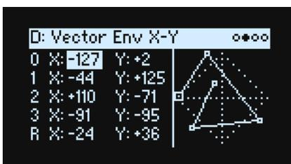
This page shows the X-Y coordinates for each point, which also translate into the Vector Env modulation outputs. You can edit these by hand if desired, or enter values into the selected point via the joystick. Unlike volumes, modulation outputs are not clipped to the diamond shape.
