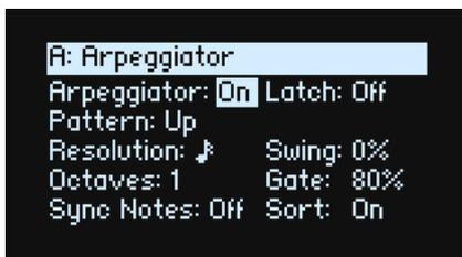
The Arpeggiator is particularly effective in conjunction with **Note Advance**, so that each generated note starts on a new step in the Lane. Try this with the Sample Lane in particular, with a single Timing step set to *Gate*.
