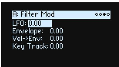
These four parameters control the default modulation routings for Filter Cutoff. You can create additional routings as desired; for more information, see “Adding Modulation Routings” on page 53.
