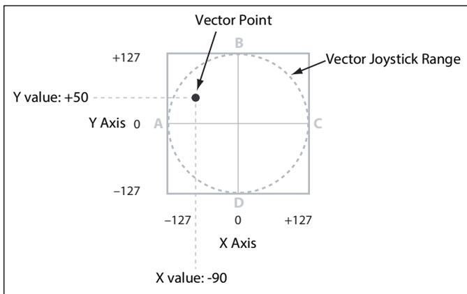
In addition to moving the point directly with the Vector Joystick, you can also use the Vector Envelope to move its position automatically over time, as shown below.
