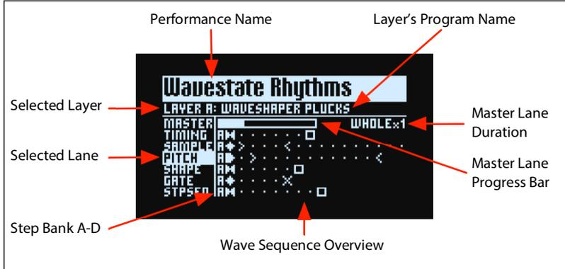
This is the wavestate’s main page, where you can select Performances, set the Layer’s Program, and see a real-time overview of the Layer’s Wave Sequence.
