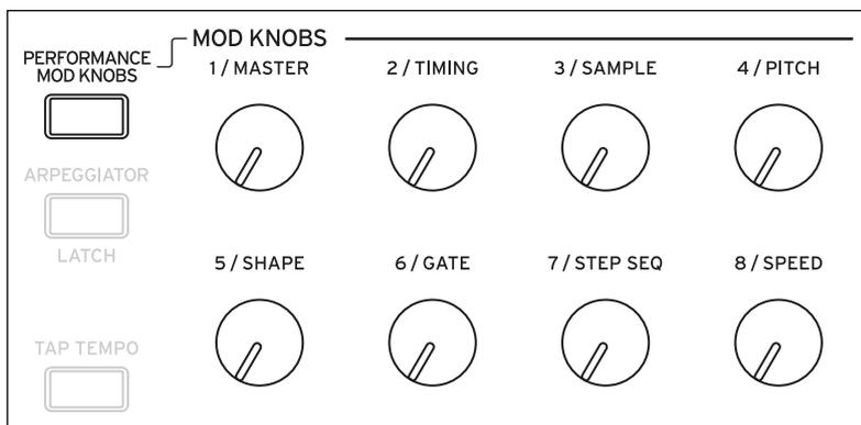
There are eight Mod Knobs per Program, each of which can modulate any number of parameters in its Program (the knob names are just suggestions). An additional layer of Performance Mod Knobs can modulate parameters throughout the entire Performance—including, specifically, the Program Mod Knobs. Each of these 40 (!) knobs sends and receives a MIDI CC; see “MIDI CC Assign” on page 84.
