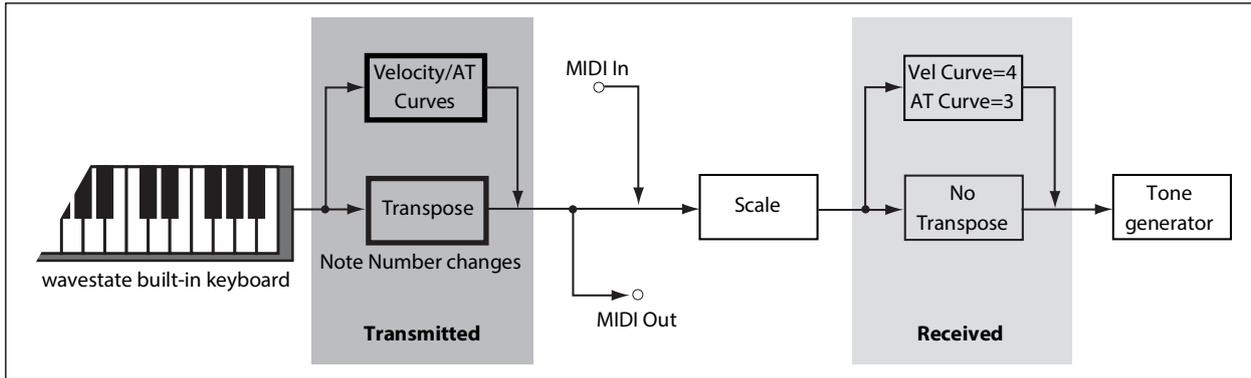
*Post-MIDI*: **Transpose** and **Velocity/Aftertouch Curves** affect MIDI *input*. Use this to adjust response to an external MIDI controller.
