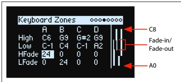
**Shortcut:** Pressing a **LAYER** button switches to the current parameter in the selected Layer's column.
