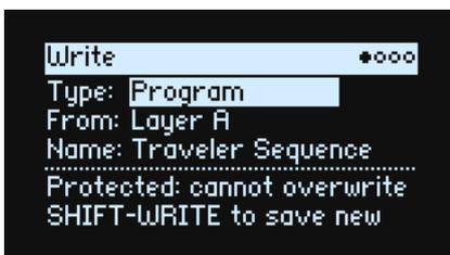
3. If necessary, set the From parameter to the desired Layer, either on-screen or by pressing one of the **LAYER** buttons.
