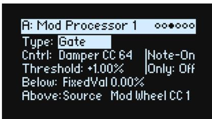
This lets you switch between two modulation sources (or fixed values) using a third modulation source.
