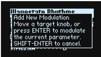
3. To select the modulation destination, move its front-panel control (e.g., **CUTOFF**), or press **ENTER** to select the parameter from step 1.
