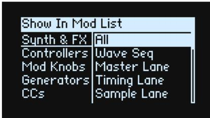
2. Press a Lane, Envelope, LFO, or Effect button; move a **MOD KNOB**; hold **ENTER** and move a controller or play a note on the keyboard (for Velocity); send a MIDI message; or for the Filter, Amp, or Pitch sections, move a knob for that section. Use the on-screen list for other selections, such as Key Track or Mod Processors.
