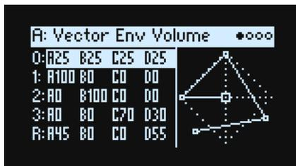
The Vector Envelope has five points: 0, 1, 2, 3 (Loop), and Release. Each point has X and Y positions, from which the A, B, C, and D percentages are derived.
