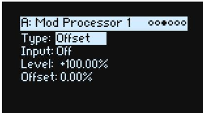
This adds a constant positive or negative offset to a modulation source, and also allows you to double the gain.
