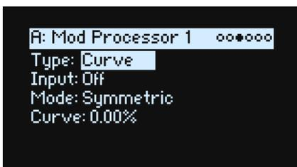
Curve can create custom controller curves, such as exponential joystick, logarithmic velocity, and so on. It can also alter the shape of programmable modulation sources, such as Envelopes and LFOs.
