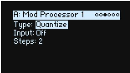
This changes a continuous signal into a series of discrete steps. Use this to change the shape of LFOs or envelopes, or to force a controller to land on a few specific values.
