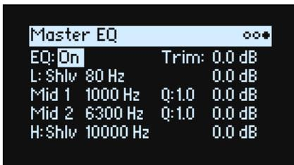
**EQ On/Off** enables and disables the EQ. Use **Trim** to compensate for EQ boosts. The **L** (Low) and **H** (High) bands can be set to *Peak*, *Shlv* (Shelving), or *Cut* (Low cut/High cut).
