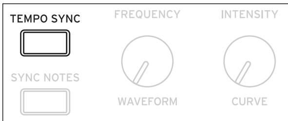
*On*: The LFO synchronizes to the system tempo, with its speed controlled by **Base Note** and **Multiply**.
