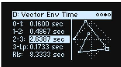
The front-panel knobs control the five Time parameters. The units are in either seconds or note values, depending on the Vector Env Setup page's **Mode** parameter.
