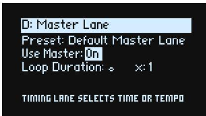
When **Use Master** is *On*, the Master Lane restarts all of the other Lanes after either a specified number of beats or elapsed time, depending on **TEMPO** On/Off (below). Unlike other Lanes, Master has no steps, so most of the front-panel Lane controls don't apply.
