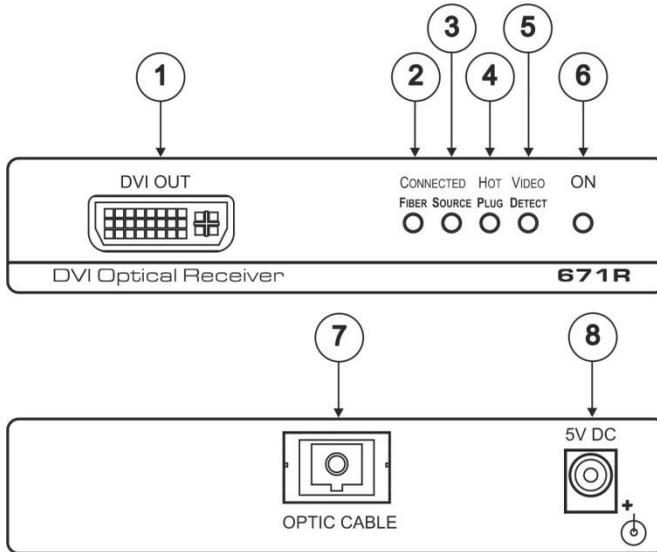
Figure 2: 671R DVI Optical Receiver
