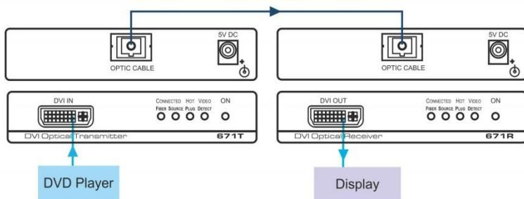
Always use Kramer high-performance cables for connecting AV equipment to the **671T, 671R**.
