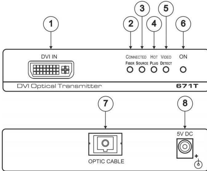
Figure 1: 671T DVI Optical Transmitter
