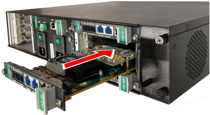
Figure 7: Input / Output Card Installation on the MTX3-16-M
