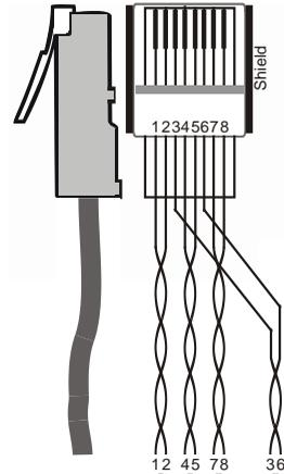
1 For a straight connection, connect pin 2 to pin 2, pin 3 to pin 3, and pin 5 to pin 5. If a shielded cable is used, connect the shield to pin 5
