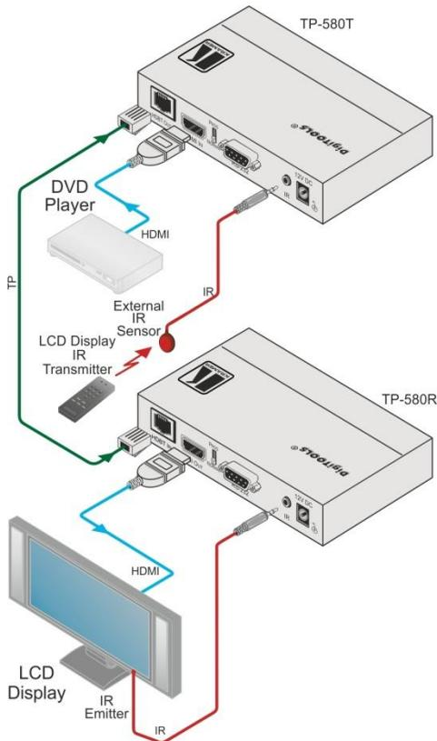
Figure 6: Controlling an LCD Display via the TP-580T
