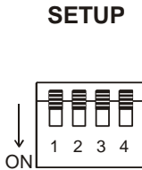
Figure 5: VS-44HDxI SETUP DIP-switches
