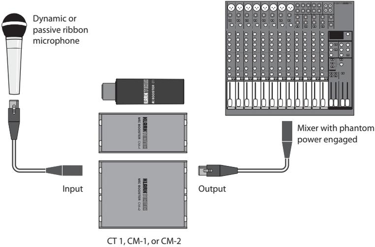
\*note – the CT 1 can also be connected directly to most microphones
