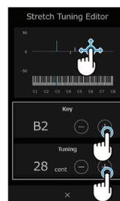
3. Tap the [-] and [+] buttons in the Tuning area to adjust the value for the selected note, or drag the graph to adjust the tuning. The Tuning value can be adjusted within the range of -50~+50 cents.
