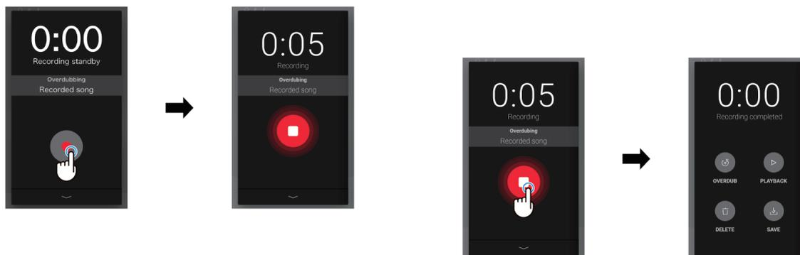
5. Tap the [Playback] button to playback the recorded performance. Tap the [Save] button to save the recorded performance, or the [Delete] button to delete it.
