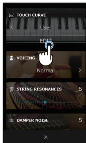
2. Select the keystroke strength from ppp to fff with the [+] and [-] buttons, or drag the graph to adjust the curve.
