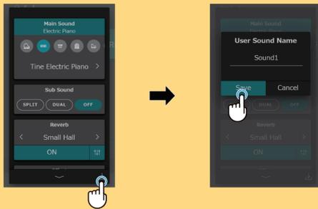
2. With the edited "Tine Electric Piano" Sound1 in this case selected, set the "Startup Screen" setting to "Sounds", and the "Startup Settings" setting to "Current".
