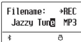
Press the ∨ or ^ VALUE buttons to cycle through the characters, and the ∨ or ^ MENU buttons to move the cursor.
