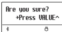
Press the VALUE  $\wedge$  button to confirm the erase operation and return to the Internal Song Player screen.
