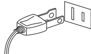
**This product shall be near the AC outlet and the power cord plug in a position so that it can readily be disconnected in an emergency because electricity is always charging while the plug is in the AC outlet even in a power switch off condition.**
