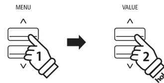
**Example:** To increase the reverb depth, press the MENU  $\blacktriangle$  button to select the “Reverb Depth” page, then press and hold the VALUE  $\blacktriangle$  button.
