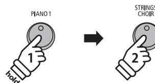
**Example:** To change the layered "String Ensemble" sound to the "Slow Strings" sound, press and hold the PIANO1 button, then press the STRINGS/CHOIR button.
