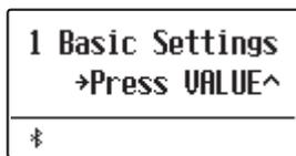
Press the  $\nabla$  or  $\wedge$  MENU buttons to cycle through the different settings menus, then press the VALUE  $\wedge$  button to enter the selected menu.
