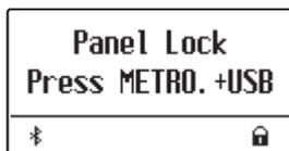
\* When activated, the Panel Lock will remain even after the power is turned off/on.
