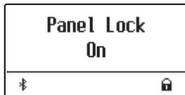
If panel buttons are pressed while the Panel Lock is activated, a reminder message will briefly be shown in the display.
