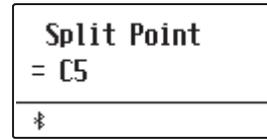
*Example: To set the split point to key C5, press and hold the SPLIT button, then press the C5 key.*
