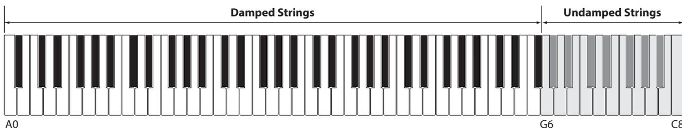
As a result, the strings of these “undamped” treble notes are free to vibrate in sympathetic resonance with those of lower keys – independently of the damper pedal position – helping to enrich the sound with additional harmonics and tonal colour.
