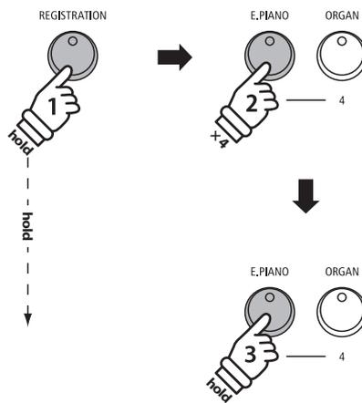
**Example:** To store the current instrument setup to memory 3D, press and hold the REGISTRATION button, press the E.PIANO button four times, then press and hold the same E.PIANO button.
