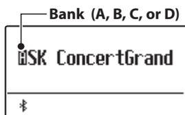
Press the SOUND buttons to select the desired registration memory. Press the same SOUND button repeatedly to cycle through the four banks (A, B, C, and D).
