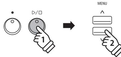
The LED indicator for the PLAY/STOP button will turn on, and the file selection screen will be shown in the display.
