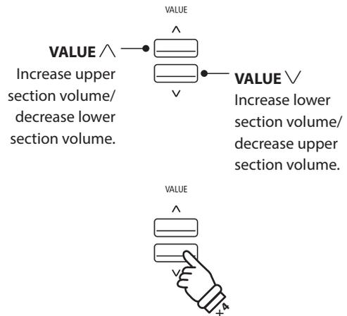
*Example: To decrease the volume of the upper section sound to 6, press the VALUE  $\nabla$  button four times.*
