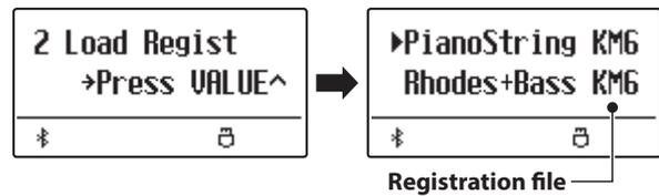
The file selection screen will be shown in the display, listing the registration files stored on the USB memory device.
