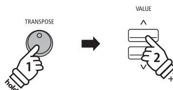
*Example: To increase the key transpose value from 0 (off) to +4 (i.e. raise the keyboard pitch by 4 semi-tones), press and hold the TRANSPOSE button, then press the VALUE  $\wedge$  button four times.*
