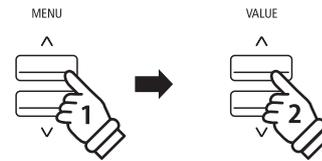
**Example:** To increase the volume of the tempo, press the MENU  $\wedge$  button to select the "Volume" page, then press the VALUE  $\wedge$  button.
