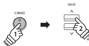
**Example:** To layer the "Classic E.P." and "60's E.Piano" sounds together, press and hold the E.PIANO button, then press the VALUE  $\wedge$  button twice.
