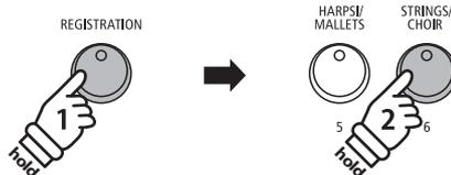
**Example:** To store the current instrument setup to memory 6A, press and hold the REGISTRATION button, then press and hold the STRINGS/CHOIR button.
