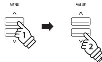
**Example:** To reduce the reverb time, press the MENU  $\blacktriangle$  button to select the “Reverb Time” page, then press and hold the VALUE  $\nabla$  button.
