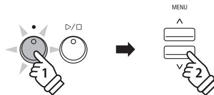
The LED indicator for the ● (REC) button will start to flash, and the USB Recorder screen will be shown in the display.
