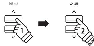
**Example:** To increase the drive of the Amp Sim, press the MENU  $\wedge$  button to select the "Amp Sim Drive" page, then press and hold the VALUE  $\wedge$  button.
