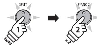
**Example:** To select the "Upright Piano" sound for the lower section, press and hold the SPLIT button, then press the PIANO2 button twice.
