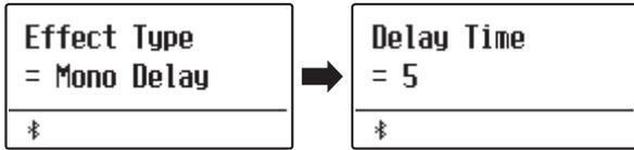
Press the  $\nabla$  or  $\wedge$  VALUE buttons to adjust the value of the selected effects setting.
