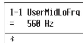
\* Frequencies set for Mid-low and Mid-high bands are applied to the second and third band equalisers from the left on the panel.
