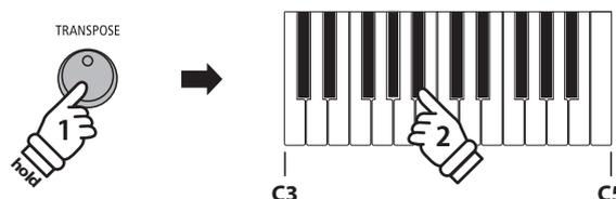
*Example: To change the key transpose from C (off) to A (i.e. lower the keyboard pitch by three semi-tones), press and hold the TRANSPOSE button, then press the A# key.*
