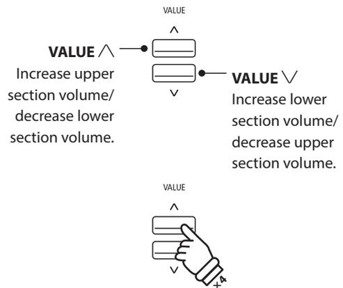
*Example: To decrease the volume of the lower section sound to 6, press the VALUE  $\blacktriangle$  button four times.*
