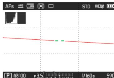
The transverse axis is indicated in level position by two green double-lines immediately left and right of the image center. When the camera is tilted, these lines are white and a short red line appears above or below them.
