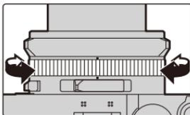
The functions that can be set with the control ring vary depending on the exposure control mode.
