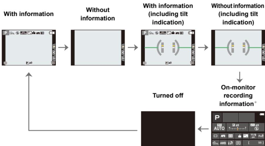
\* Displayed when [Monitor Info. Disp.] in the [Custom] ([Monitor / Display]) is set to [ON]. You can touch the desired item and change its setting directly.
