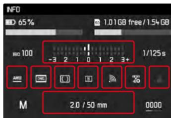
In addition to providing an overview of the most important settings, the status screen also allows quick access to specific menu functions.
