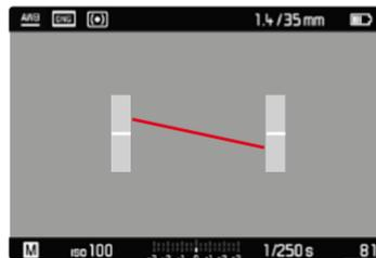
The longitudinal axis is indicated in zero position by two short lines in the gray bars to the left and right of the image center.
