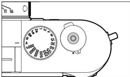
The shutter button works in two stages.
