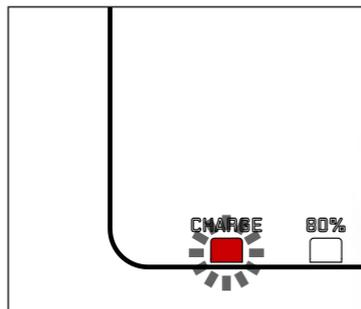
The status LED indicates a correct charging process.
