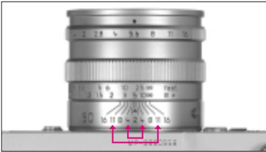
For example, if the LEICA SUMMILUX-M 50mm f/1.4 lens is set to 5m, the depth of field at f/4 is from approximately 4m to 8m. If you then stop down to f/11 with the same distance, the depth of field is from 3m to around 20m.
